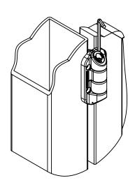
Rotate the cam clockwise to increase (+) spring tension. To decrease (-) spring tension, press the wrench downward, pushing the cam into the barrel, and rotate the cam counterclockwise. Adjust one hinge at a time in 1/4 turn increments.
