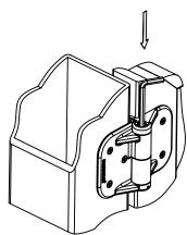
Rotate the cam clockwise to increase spring tension and counter-clockwise to reduce spring tension. Adjust one hinge at a time in 1/4-turn increments.
