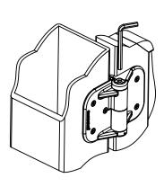
Press the wrench downward, pushing the cam into the barrel.
