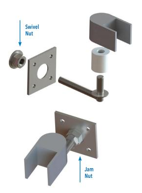
The Heavy Duty Estate Gate Hinge features a swivel nut which allows the installer to make horizontal adjustments without having to remove the gate.
