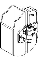
Rotate the cam clockwise to increase (+) spring tension. To decrease (-) spring tension, press the wrench downward, pushing the cam into the barrel, and rotate the cam counterclockwise. Adjust one hinge at a time in 1/4 turn increments.
