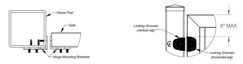
STEP 2. Install self-closing hinge assembly to mounting brackets (installed in step 1) and secure with acorn nuts (USE HAND TOOLS ONLY). Hinge should be positioned as shown so that the locking grooves on the mounting flanges will align with grooves on the back side of the hinge assembly. This will allow the hinge to be adjusted horizonally on the gate side, and vertically on the post side.
