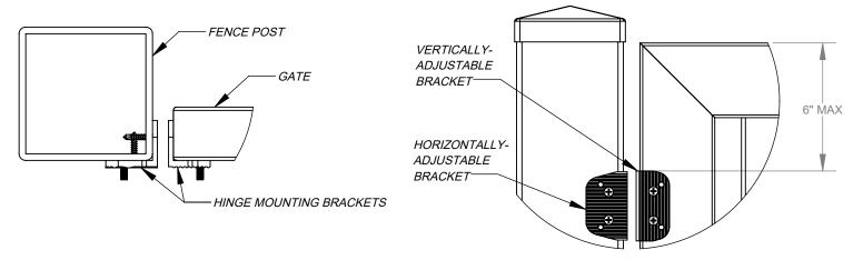
STEP 2: Install the outer hinge assembly to the mounting brackets and secure with acorn nuts using hand tools only. The hinge should be positioned as shown so the locking grooves on the brackets align with the grooves on the back of the outer hinge assembly.
